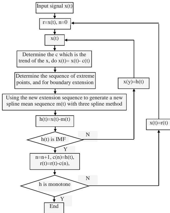
FIGURE 3 The steps of improved EMD method
