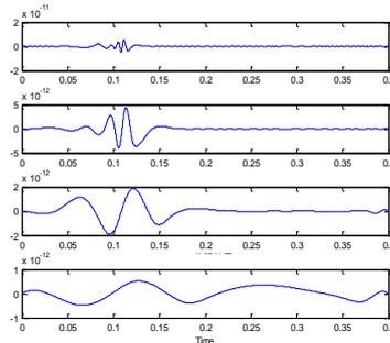
FIGURE 7 Applying the improved EMD to decompose normal signals
