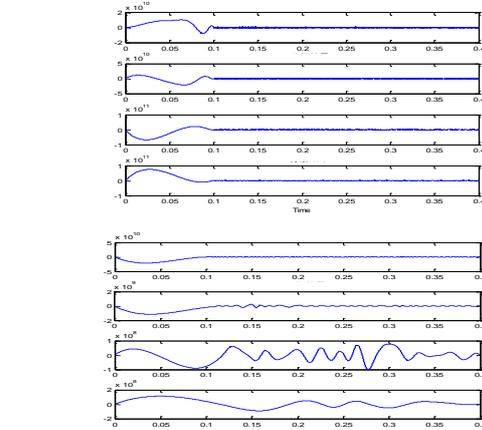
FIGURE 8 Applying the improved EMD to decompose loosening signals
