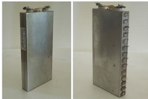
(a) Physical photo of steel shell LIB
