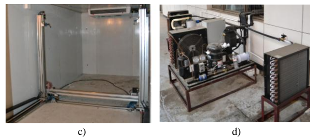
FIGURE 4 The refrigerated truck experimental platform: a) Maintenance structure, b) Environment simulation room, c) Automatic test system, d) Refrigeration and heating equipment.
