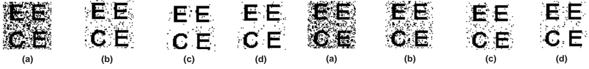
Figure 8. Recovered watermark from lenna after JPEG compression attack
