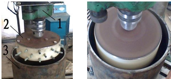
1) Drill 2) Finishing parts 3) Workpiece FIGURE 7 Photos of experimental device and finishing status
