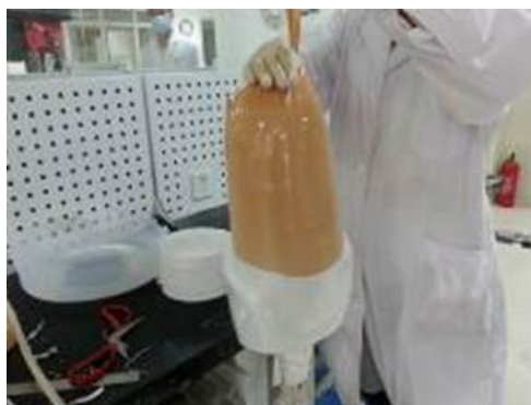
FIGURE 6 Shaping and molding process of prosthetic sockets based on carbon fibre-reinforced plastic materials.
