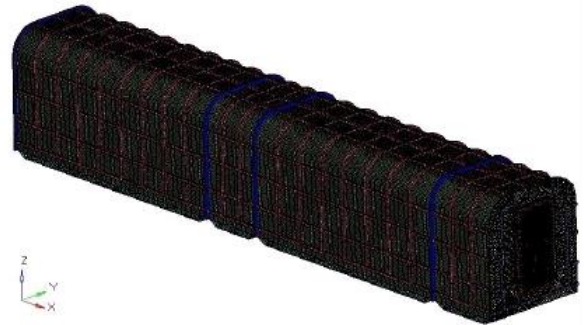
FIGURE 1 KJYF-96/8 mine mobile hardware capsule mesh model
