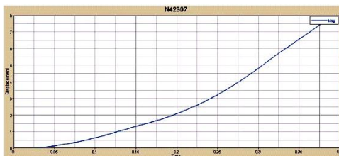
a) Peaks at 0.6 MPa, the capsule reach maximum displacement of the nodes of the \delta -t curve
