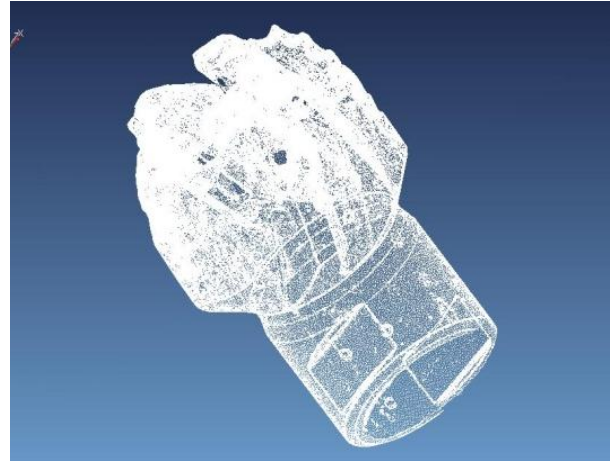
FIGURE 3 The point clouds of roller bit before reducing
