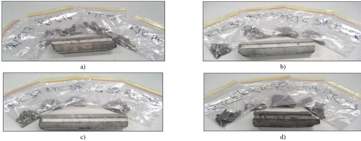
FIGURE 2 Sandstone samples and rock-cutting debris: a) No. 377542, b) No. 377554, c) No. 370526, d) No. 377590
