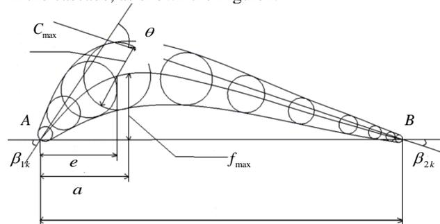
FIGURE 1 Main geometric parameters of the blade
