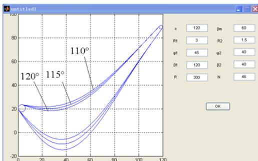
FIGURE 7 Air intake angle effects on type line of blade
