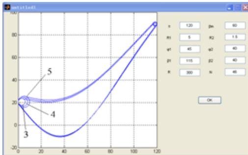
FIGURE 4 Effect of leading edge radius on type line of blade
