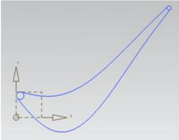
FIGURE 9 Type line of single blade cross-section
