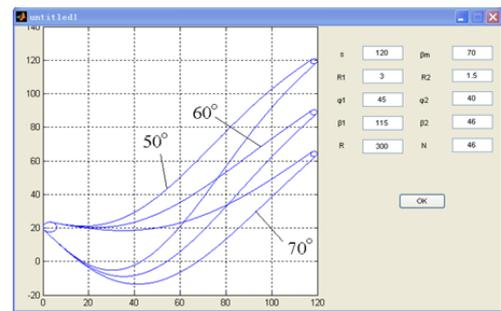
FIGURE 5 Effect of Installation angle on type line of blade
