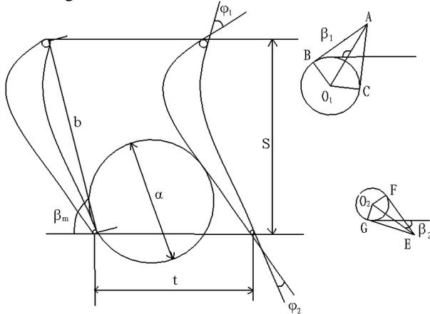
FIGURE 2 Main geometric parameters of blade cascade
