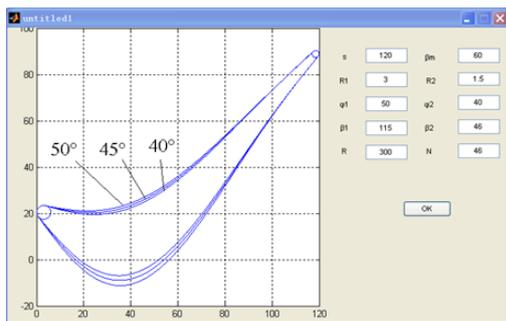
FIGURE 6 Angle of the intake side effects on type line of blade
