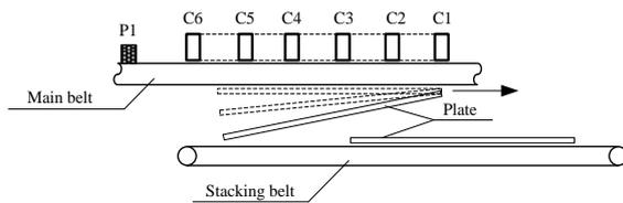
FIGURE 5 dropping control schematic diagram of 1# stacking table magnetic system
