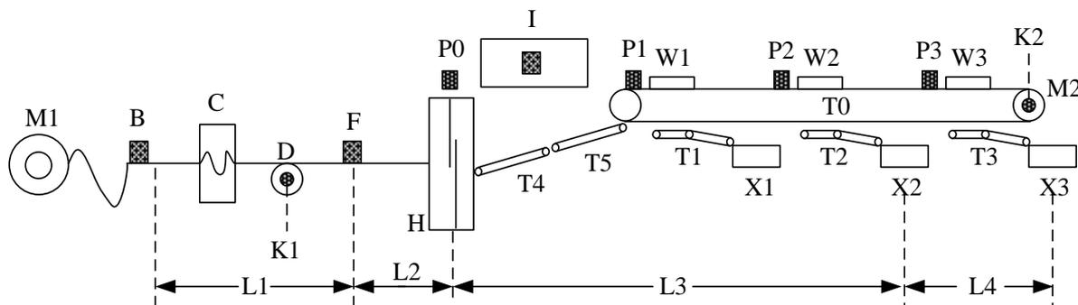
FIGURE 1 Sheet sorting system process flow
