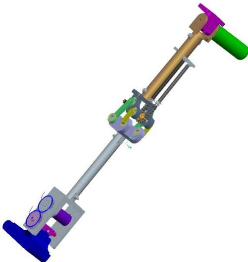
FIGURE 14 Virtual prototype of artificial leg
