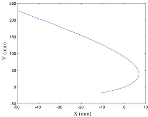
FIGURE 6 ICR of 4-bar multiaxial knee joint.
