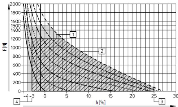
FIGURE 13 The characteristic curves of FESTO-MAS-20-200N-AA-MC-O-ER-EG
