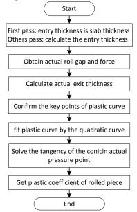
FIGURE 4 Calculation diagram of plastic coefficient
