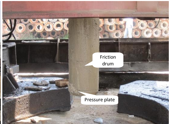
FIGURE 2 The field test of model pile.
