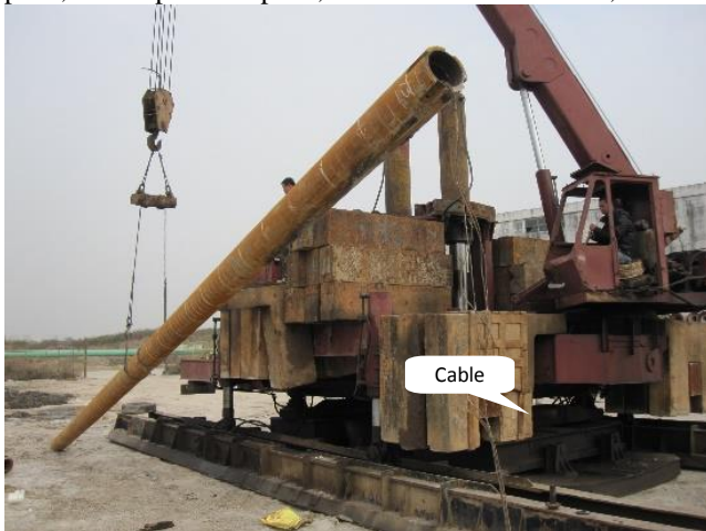
FIGURE 2 The field test of model pile.
