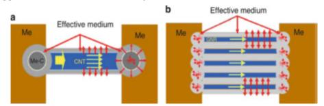
FIGURE 1 Models of C-Me interconnects as a prototypes of novel nanodevices: (a) CNT- Me interconnect; (b) multilayered GNR-Me interconnect
