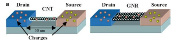
FIGURE 2 The unperturbed field-effect transistors based on a CNT and GNR are given CNT- or GNR- based FET. They are mainly composed of a corresponding semiconducting carbon material suspended over two electrodes
