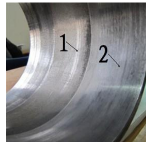
1) before finishing 2) after finishing FIGURE 9 Contrast photos before and after finishing
