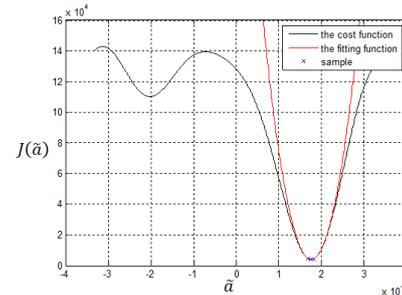
FIGURE 2 The fitting of the cost function of one OFDM block
