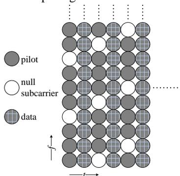
FIGURE 1 Illustration of pilot and null subcarrier pattern
