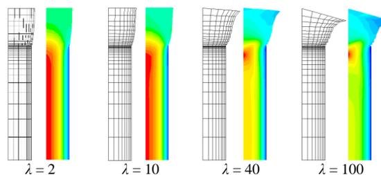
FIGURE 6 The contour map of meshing grid and Y-axis velocity in different relaxation times
