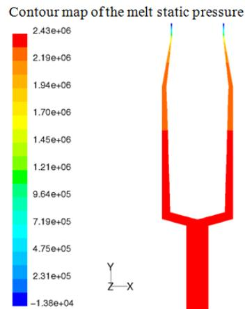
FIGURE 4 contour map of the melt static pressure
