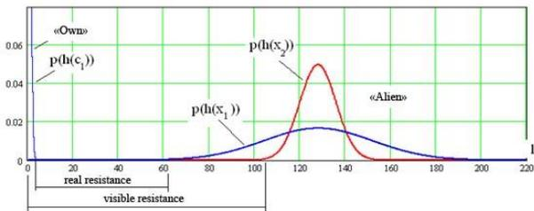
FIGURE 6 Compression of the Hamming distance distribution at the output of neurons of the second layer due to the hashing properties of neurons
