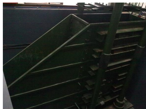
FIGURE 4 The side slope tunnel coupling experiment system
