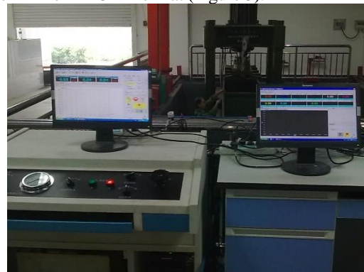
FIGURE 3 The microprocessor control electro-hydraulic servo tester's measurement and control system
