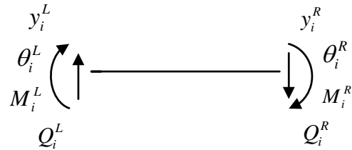
FIGURE 3 Force analysis diagram for i^{\text{th}} span
