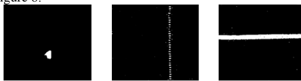
FIGURE 8 Threshold segmentation image of defects
