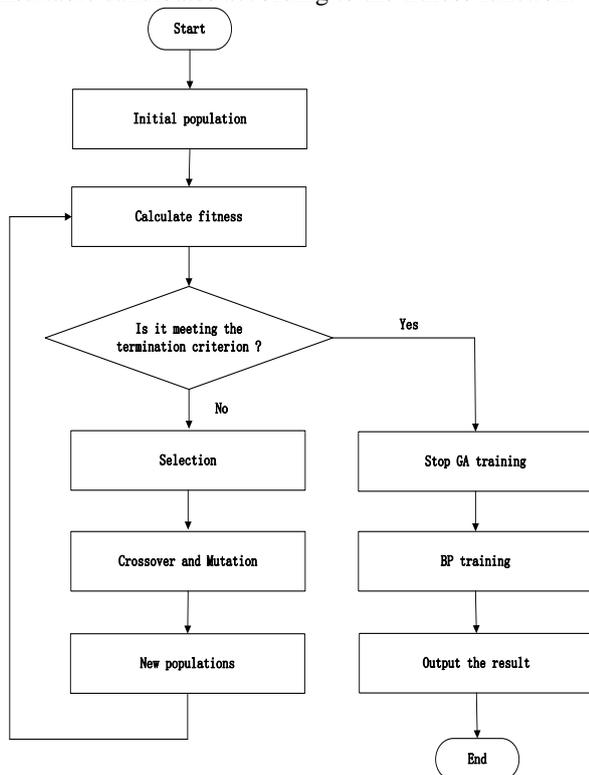
FIGURE 1 Framework of training a neural network using GA
