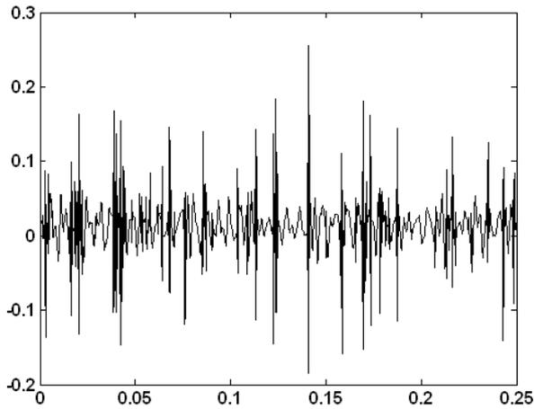
FIGURE 3 The de-noising signal of outer ring fault
