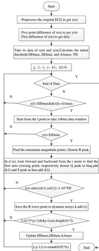
FIGURE 9 The R wave detection process
