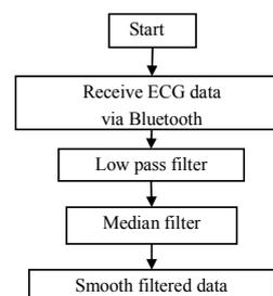
FIGURE 1 The flow diagram of signal filtering
