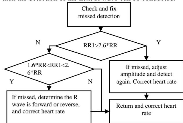
FIGURE 11 The process of R wave detection missed
