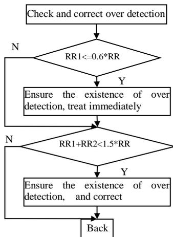
FIGURE 10 Over-detection process
