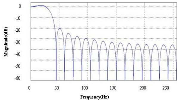
FIGURE 2 The low-pass filter characteristics
