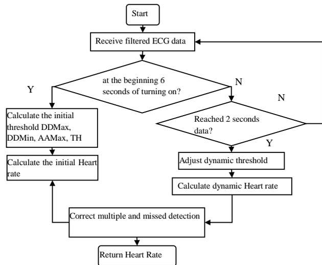
FIGURE 8 Heart rate calculation flowchart
